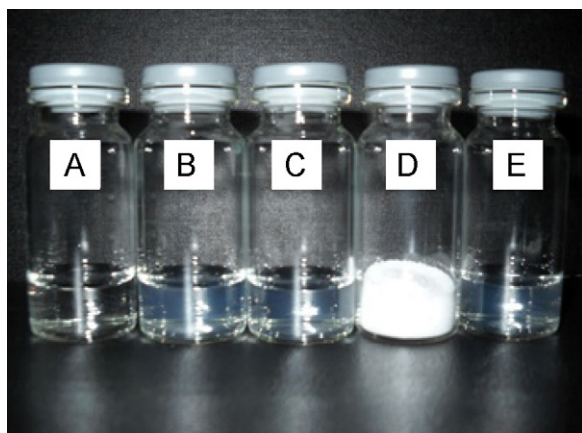
Fig. 2. Morphology of PTX-loaded PCEC micelles: (A) water; (B) PTX–PCEC micelles; (C) PTX–PCEC–P80 micelles; (D) freeze-dried powder of PTX–PCEC–P80 micelles; (E) the re-dissolved PTX–PCEC–P80 micelles in normal saline.
